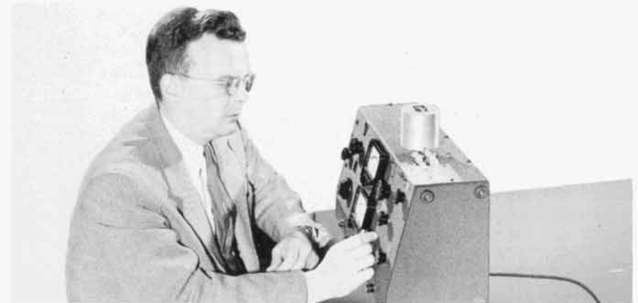
Figure 1. The author measuring the dissipation factor of Teflon.
